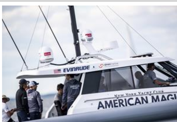
KVH's TracPhone V3-HTS and TracPhone LTE-1 are installed on American Magic's chase boat, providing data transmissions.
