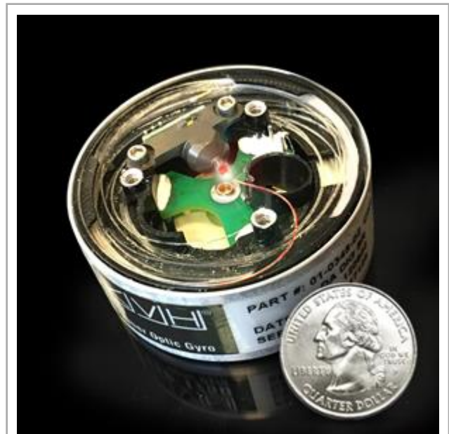
KVH's extremely small, high-precision fiber optic gyro (FOG) is key to a driverless car's performance. In this photo, the red illumination represents light moving through the FOG's optical circuit of coiled fiber; this circuit is the FOG's sensing unit—it is mounted with power and processing electronics within a driverless car to provide precise data for the car's navigation systems. The quarter indicates the sensor's relative size.
